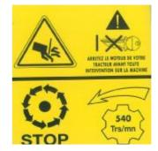
Stop the tractor engine and remove the key before working on the machine.
